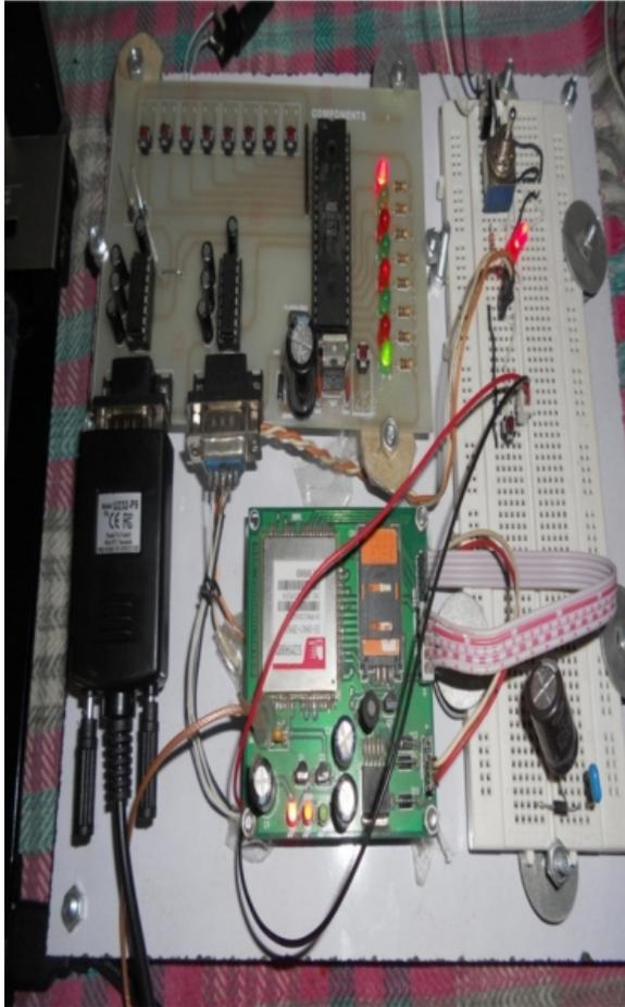
Fig. 4. Hardware module for sending SMS on unauthorized access
