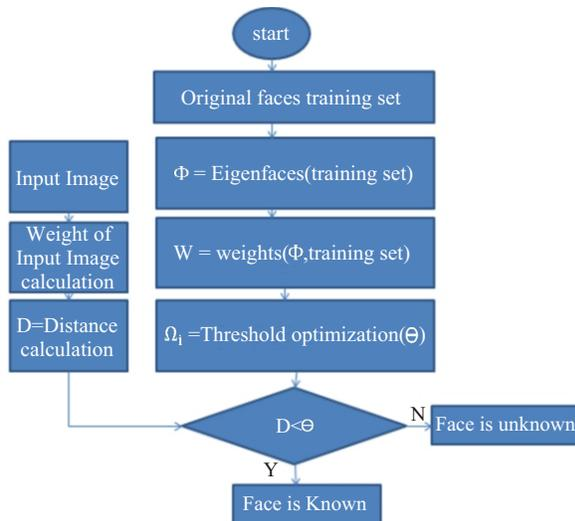
Fig. 7. Flow chart for threshold optimization
