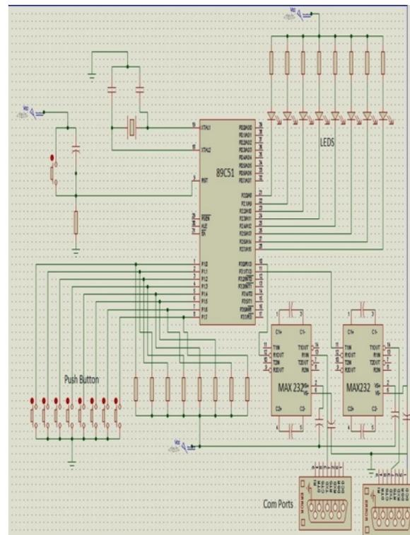
Fig. 3. Schematic diagram showing interfacing of different components
